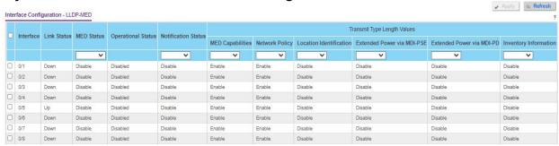
The **Link Status** field displays the link status of the port (up or down).
