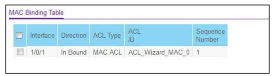
To delete a MAC ACL-to-interface binding, select the check box next to the interface and click
